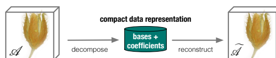
Figure 1: Compact data representation for a 3 rd -order tensor \mathcal{A} (a volume) by bases and coefficients that can be used to reconstruct the data to its approximation \tilde{\mathcal{A}} at run-time.
