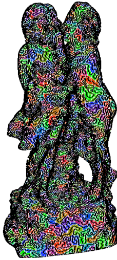
Figure 1: Single cycle triangulation of the genus-two sculpture model with 50780 input and 51780 output triangles.
