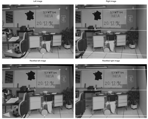
Fig. 5 “Sport” stereo pair (top) and rectified pair (bottom). The right pictures plot the epipolar lines corresponding to the points marked in the left pictures.
