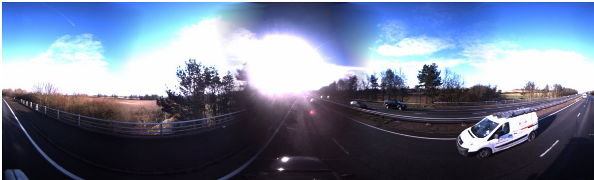
Fig. 19: The two highest confidence false positives in the 1,000 km data set. Both matches are assigned probabilities very close to 1. In (a), we pass a similar-looking roundabout. The locations are 1 km apart. In (b), we encounter the same van twice. The locations are 9 km apart. Such rare-but-repetitive objects represent the most challenging class of perceptual aliasing.
