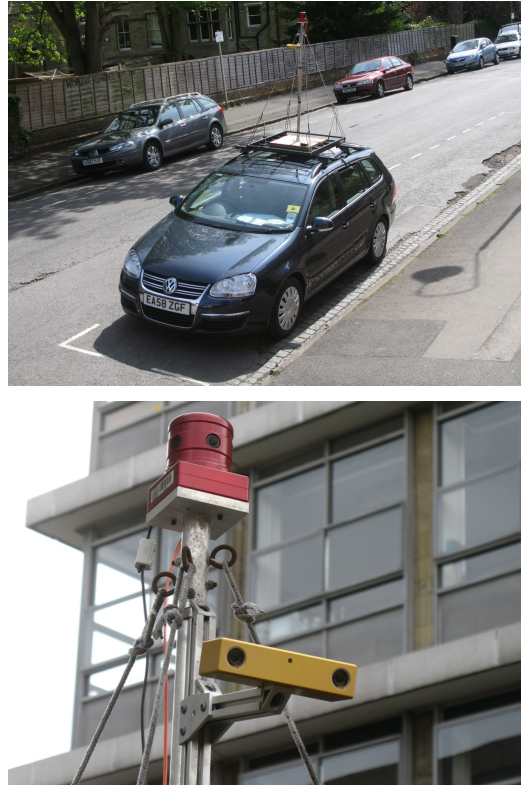
Fig. 8: Vehicle and sensor rig used to capture the 70 km and 1,000 km data sets. The rig consists of a Ladybug2 omnidirectional camera and Bumblebee stereo camera, both from Point Grey Research. The cameras were mounted approximately three meters above the road surface. GPS data was collected with a Seres unit from CSI Wireless, mounted on the roof of the car.
