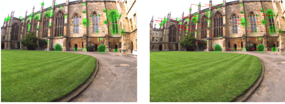
Fig. 5: A example of geometric verification, showing inliers identified by RANSAC. Note that we are not recovering an exact pose-to-pose transformation; the correspondences are only approximately geometrically consistent.
