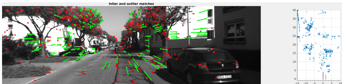
Figure 1: Outlier rejection and localization using PNP and RANSAC. Left: Inliers with displacement (green) and outliers (red). Right: 3D points (blue) and recovered camera poses.
