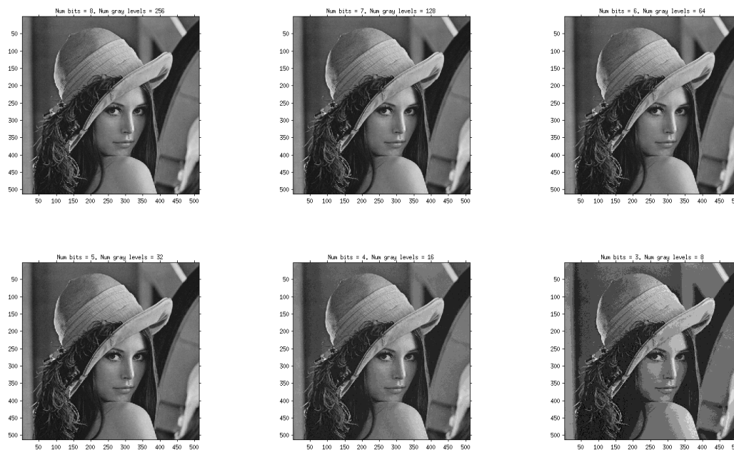
Figure 4: Effect on image quality of reducing the intensity resolution of the image, i.e., the number of gray levels used to represent the underlying continuous intensity signal.
