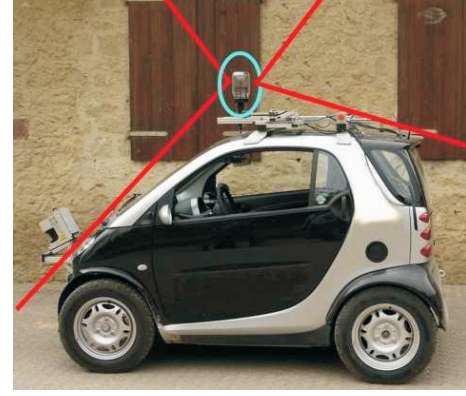
Fig. 9. Our vehicle equipped with the omnidirectional camera. The field of view is highlighted.
