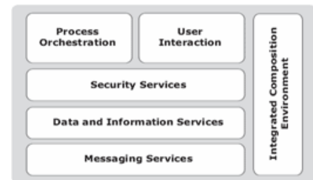
A typical ESB stack
