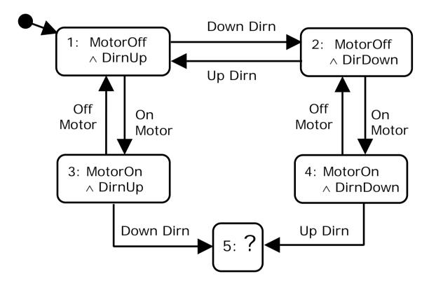
• Dirn must not be switched while the motor is on
