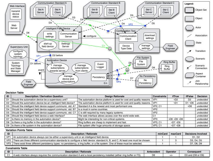
Figure 1. The automation device product line specified in the ADORA language.
