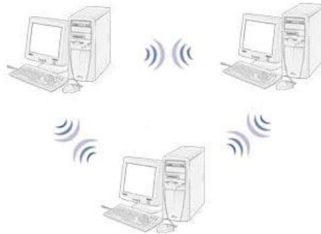
Figure 8.3: Ad-Hoc-Installation
