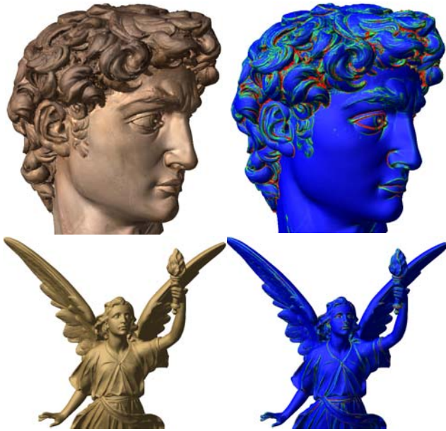
Figure 16. Results of applying normal computation and splat estimation; and curvature stream operators to raw point cloud data sets. The left column shows the high-quality normal estimation and on the right the qualitative (RMS) curvature strength is color coded.
